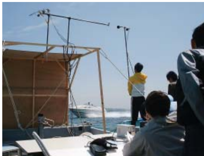
Test for measurement of noise emission
