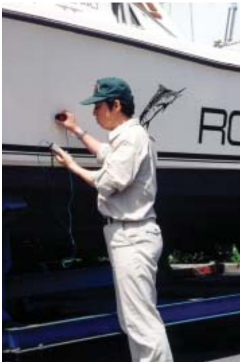
Measurement of hull thickness
