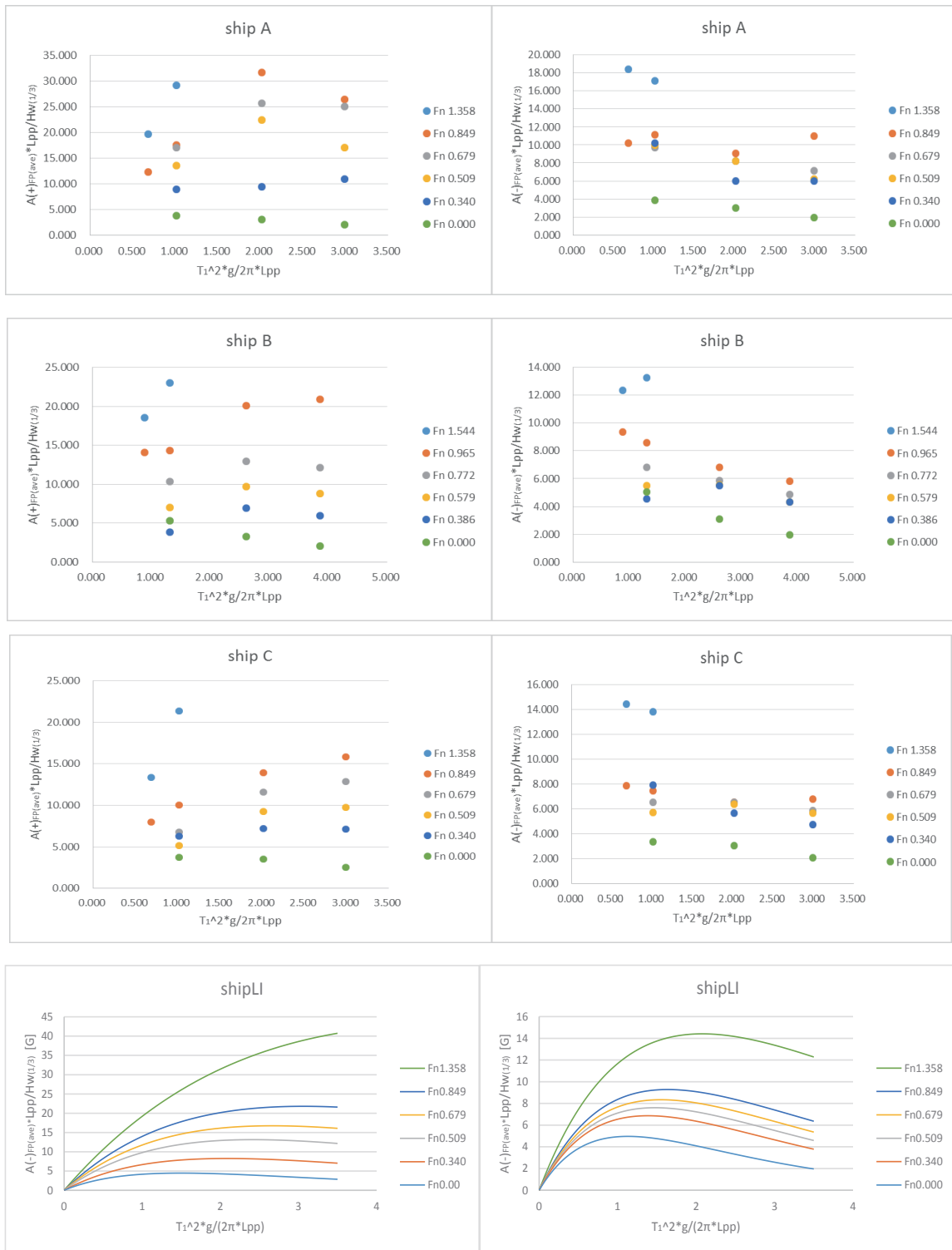
Fig.4-2-37 Measured non-dimensional average upward or downward peak value of vertical acceleration on hull obtained by Eq.4-2-24 for Ship A, Ship B and Ship C. The data of Ship LI obtained from linear interpolation between measured acceleration of Ship A and that of Ship B for L_{pp}/B . Ship LI is L_{pp}/B=4.11 .
