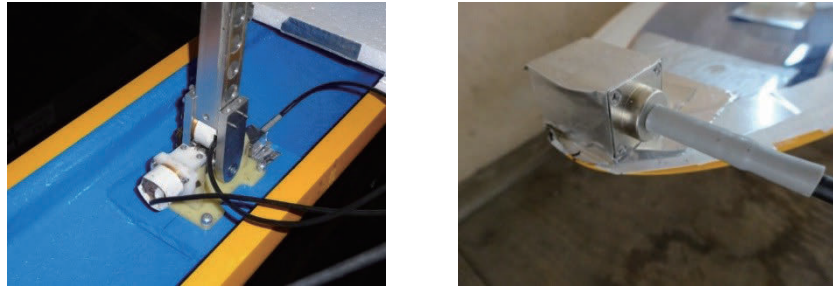
Fig.4-2-4 Pictures of motion measuring device and acceleration center (KYOWA ASW-20A).
